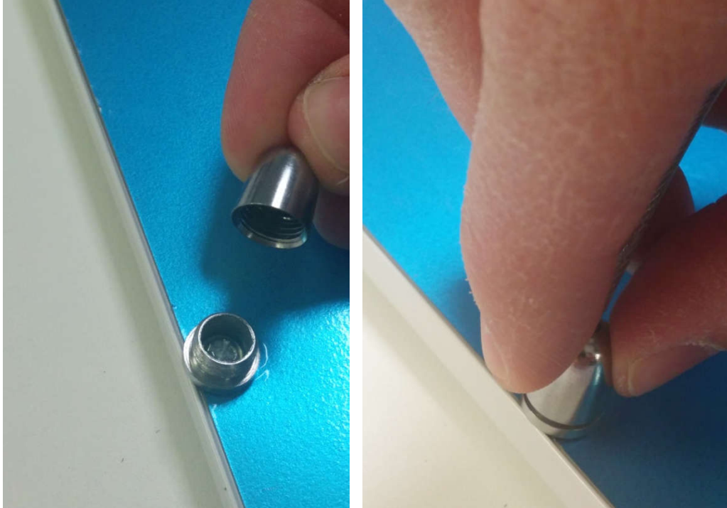
Screwing the suspension piece into the cylinder-screw
